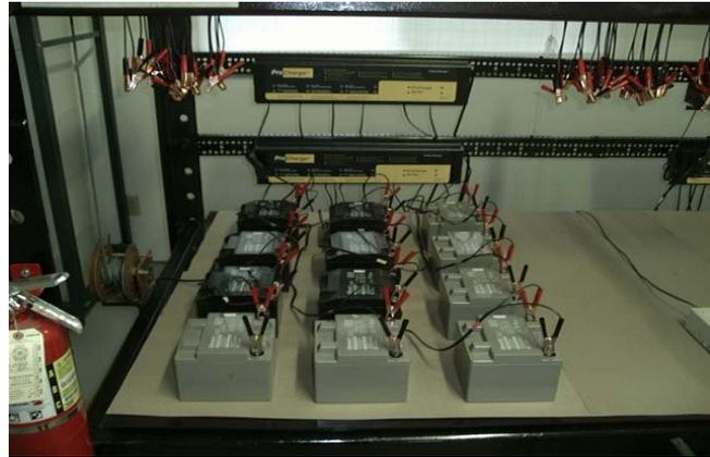
Automated 12 Volt Battery Charging System designed to charge and maintain up to six batteries at a time. Each station operates separately. With an optional lead set, the system charges and maintains up to 12 batteries at 2.5 amps and 36 batteries when three stations are connected together.
